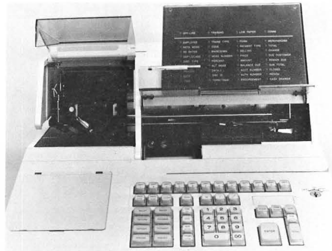
The TRW-Fujitsu Company's 7880 POS System is said to be the first on the market to offer as options such state-of-the-art technology as bubble memory, plasma display, and an integrated magnetic stripe card reader.
