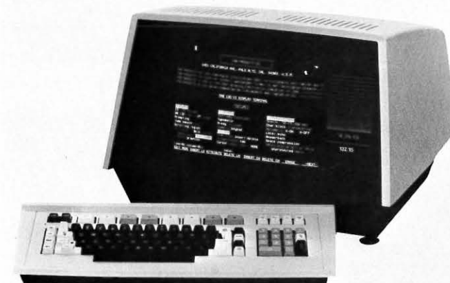
The TAB 132/15 Smart Display Terminal features a 15-inch, high resolution, non-glare screen, with 80 or 132 column format. Large, flicker-free characters are formed by a 7 x 11 dot matrix in a 9 x 14 or 9 x 16 cell. Character attributes include blinking, bold, underline, reverse video. Protected fields may be based on any attribute.
